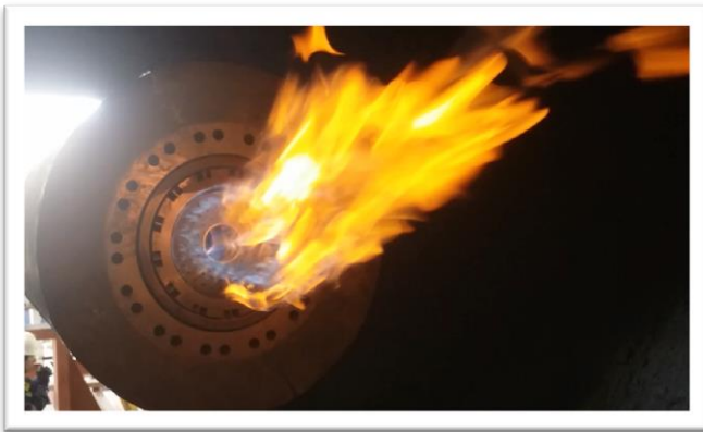
Example of a gas premix flame on a Pillard Novaflam ® burner installed on a clinker kiln
