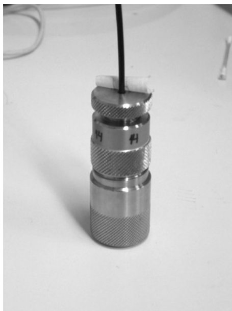
Figure 4: Bottle closure permeability measurement device.
