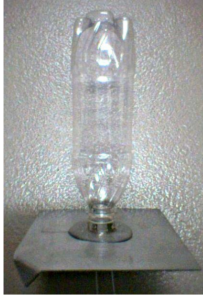
Figure 1: Oxttran bottle mounting set-up.
