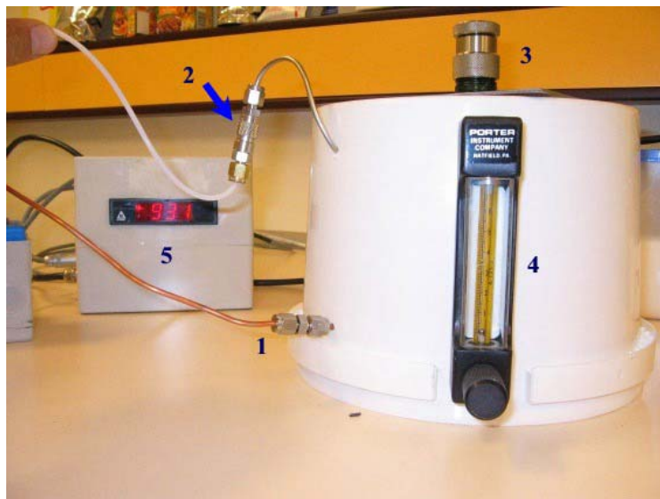
Figure 3: Calibration set-up showing gas inlet (1), pressure transducer connection (2), bottle closure holder (3), and flowmeter (4) permitting pressure control for the calibration and pressure display (5).
