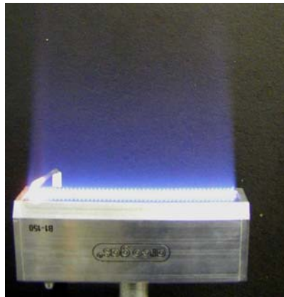
Fig.2: Example for a flame of a burner used for treatment of even surfaces like films, foils, paperboards.
