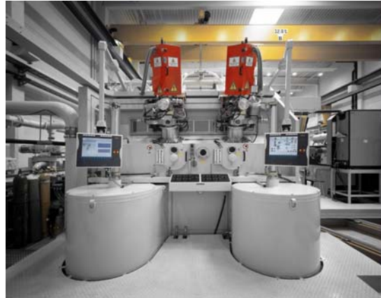
Fig. 6 Electron beam system with two guns, 2,1 m coating width ( TOP BEAM-Applied Materials).
