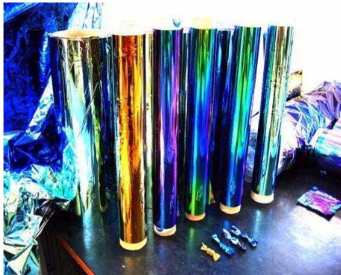
Fig. 4 Various colors created using the Fabry Perot layer system on a PET film ( e.g. Al- \text{Al}_2\text{O}_3 -Al).
