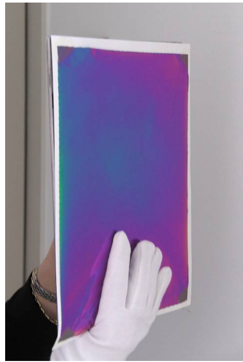
Fig. 3 Fabry Perot Layer with green color ( 0^\circ ), and turned to 45^\circ changes to blue color.
