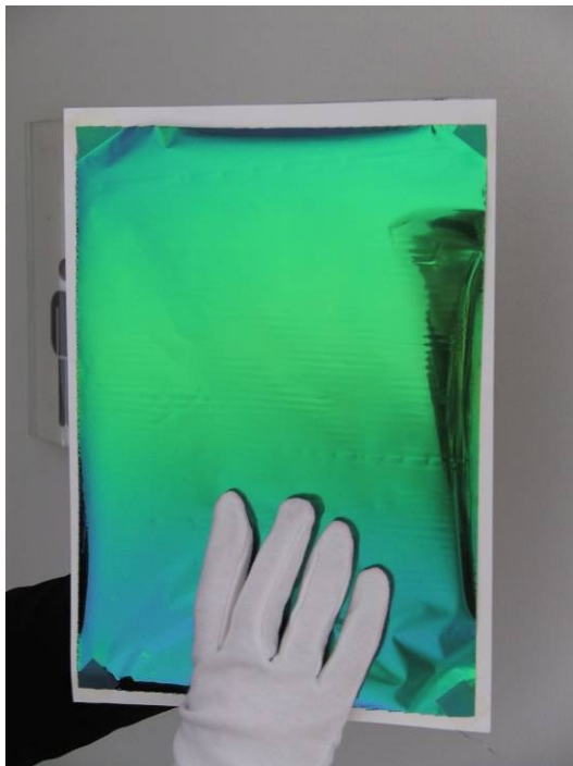
Fig. 3 Fabry Perot Layer with green color ( 0^\circ ), and turned to 45^\circ changes to blue color.
