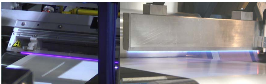
Figure 1. Corona treatment (on the left side picture) and flame treatment (on the right side picture).
