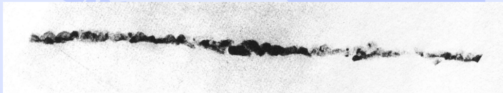
Metallized, plain PET film Metal penetration = 30-40Å
