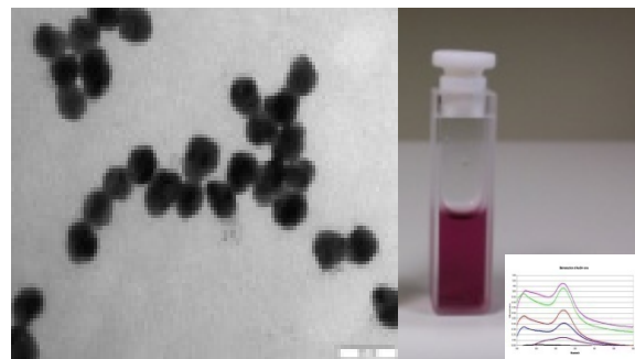
TEM image of biogenic AuNPs ~30nm (left) and AuNPs in solution (right). Inset: absorption spectra of AuNP in solution over time.
