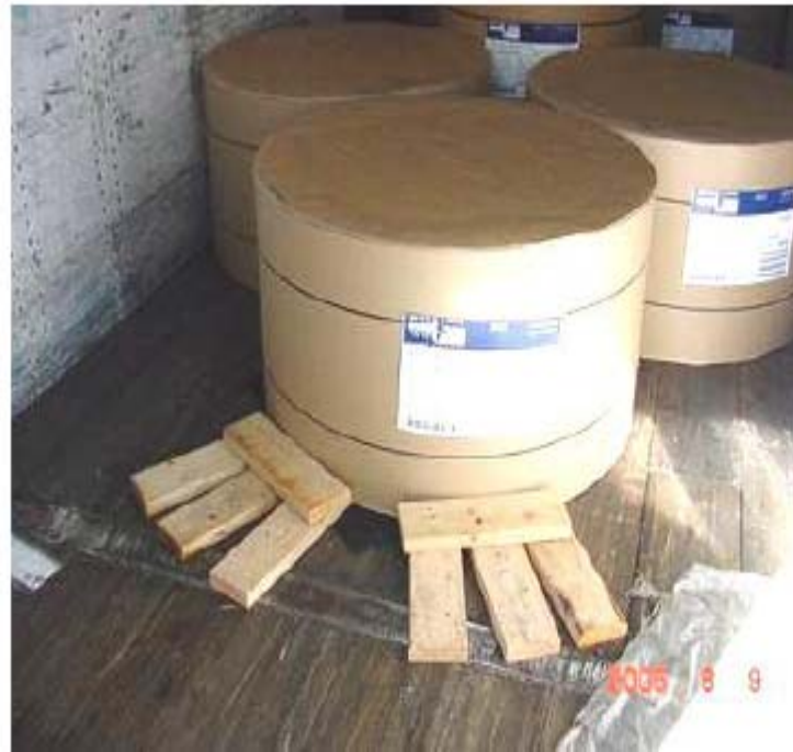
LAMINATED 2" X 6" X 24" E-BRACES. 2 PER REAR POINT ROLL
