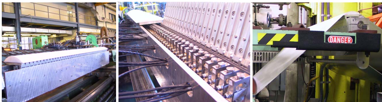
Figure 1: The new tension beam installed on the lathe during its fabrication (left), inside view of the 50 load cells (center) and the beam in operation with paper on it (right).
