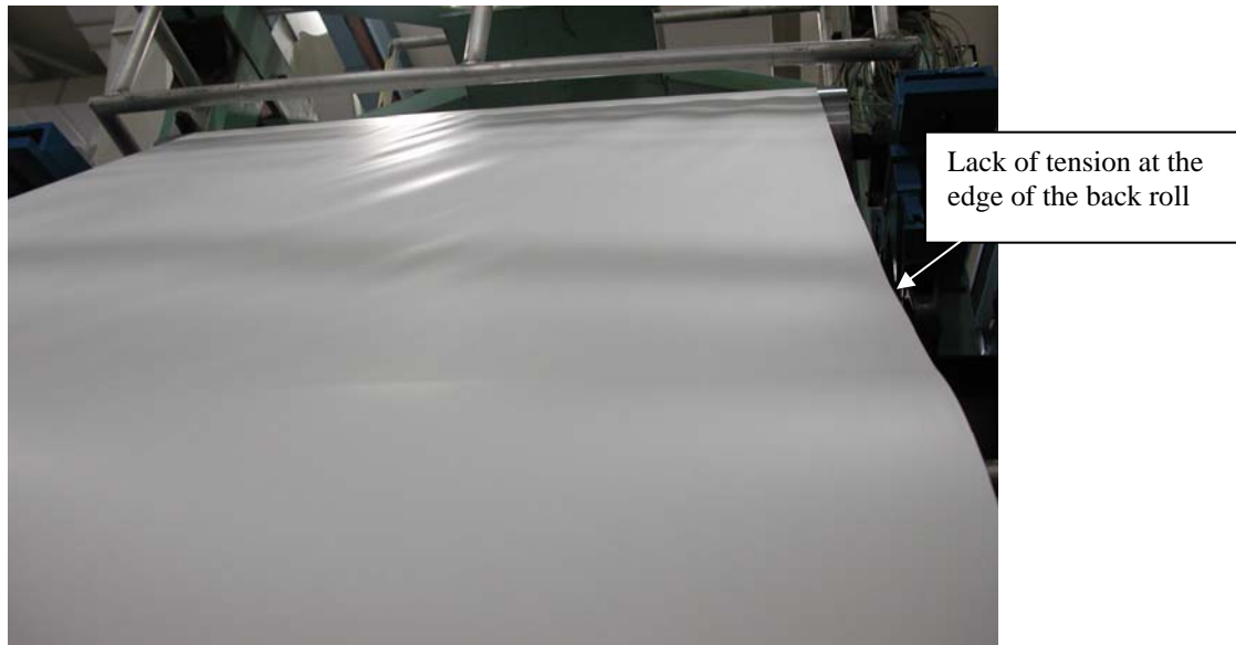
Figure 4: Case study 1 - Baggy edge problem at the back of the machine is clearly shown here at the unwind station of the roll tester
