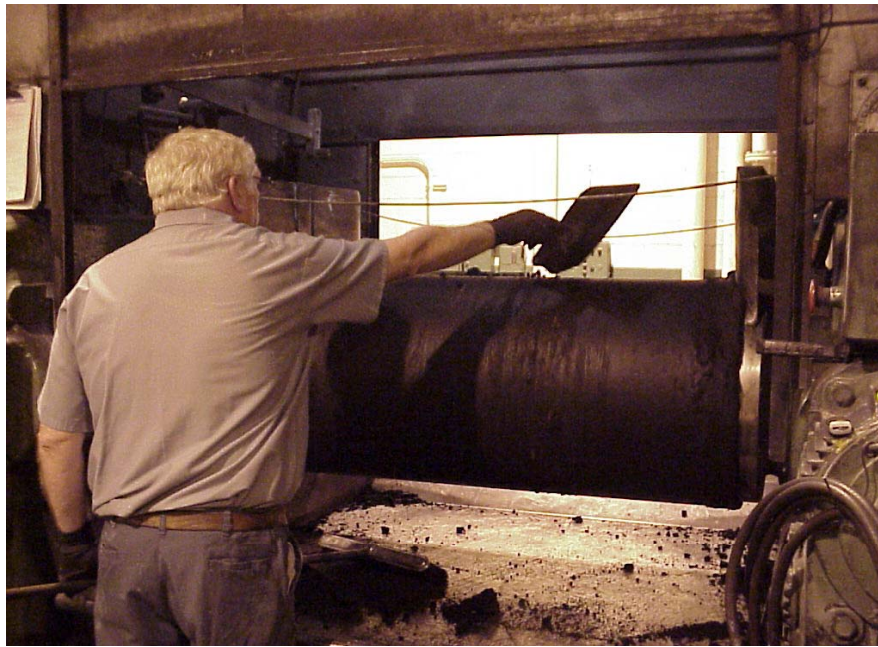
2-roll mills to blend rubber components
