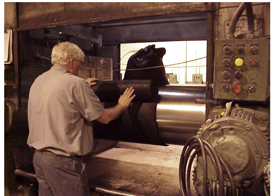
2-roll mills to blend rubber components
