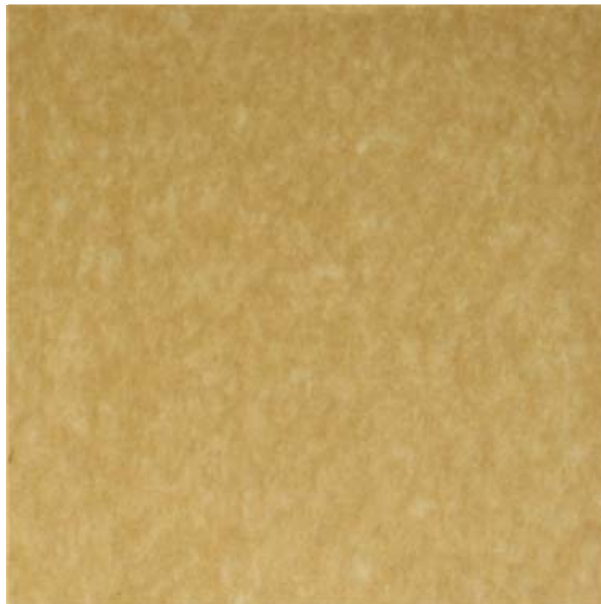
Figure 5B. Poor layer coverage produced using a conventional two-layer headbox.
