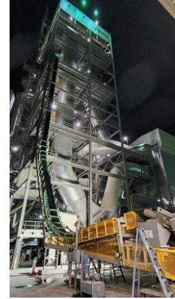
Hybrid Sandwich Belt conveyor transports rejected tires to fuel a cement plant.
