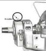
Figure 14 – Breather location on a typical Goulds double suction pump. Image courtesy of Goulds Pumps.
