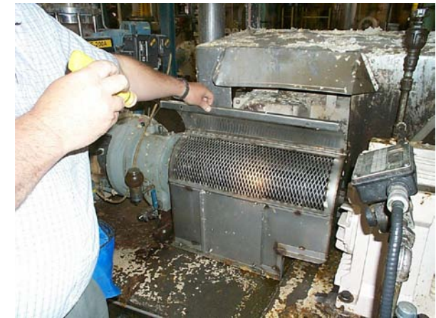
Belt and Coupling Condition with Stroboscope
