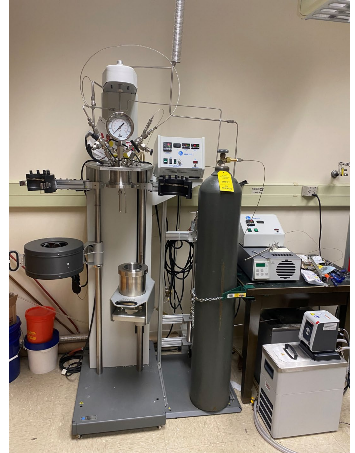
New Supercritical Fluid Deposition System 40 g CNF/PLA
