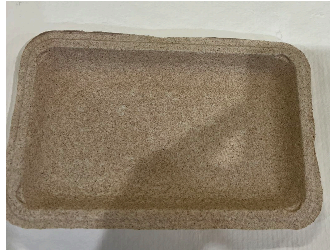
Wood flour (WF) plate with CNF as a binder
