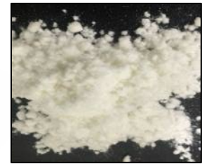
Dried, modified CNF ready for melt compounding
