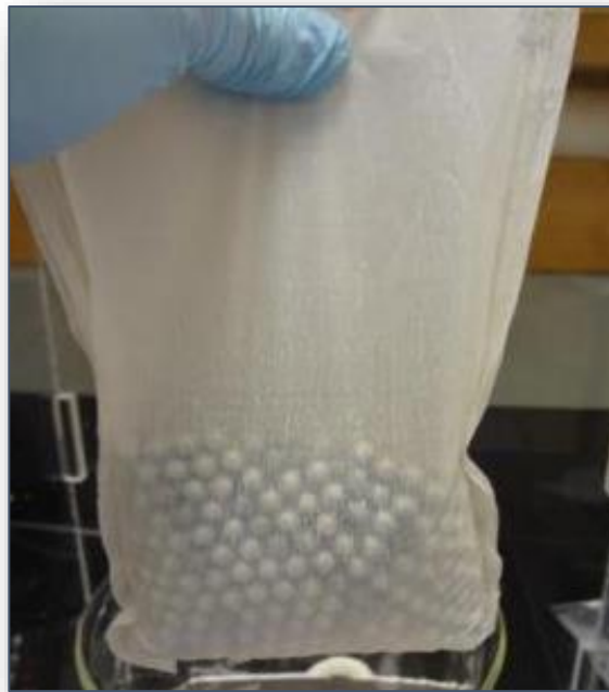
Heat-sealed CF film carrying a load >1.3 kg
